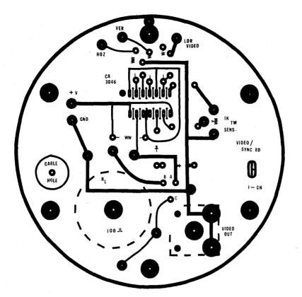
Fig. 14. Foil side of video/sync board.
