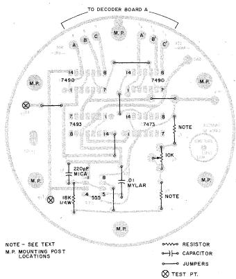
Fig. 4. Component side of LDR board. M.P. designates mounting post (threaded spacer) locations. Use alternate locations between any board pair, thus only three spacers looking like a triangle between any board pair. Small circles are socket pins for LDRs. Solid dots are leads from decoder board B and should be inserted and soldered from the copper side and excess lead on component side clipped off flush with board. Resistor symbols are LDR locations.
