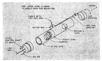
Fig. 16. Mechanical assembly of the camera.
