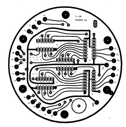
Fig. 8. Foil side of decoder board A.
