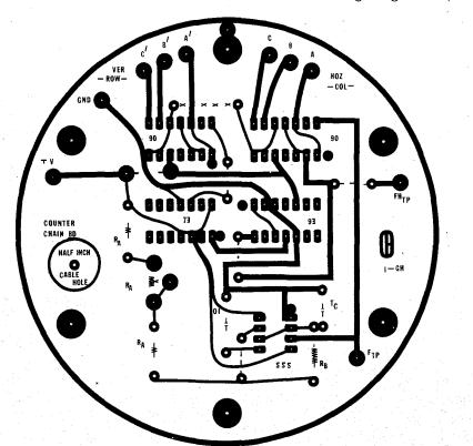
Fig. 5. Foil side of counter chain board. 73 Magazine • February, 1982
