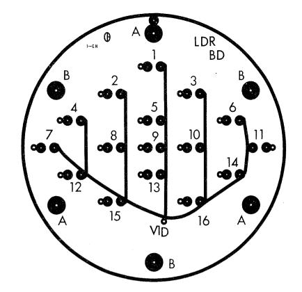
Fig. 2. Foil side of LDR board.
