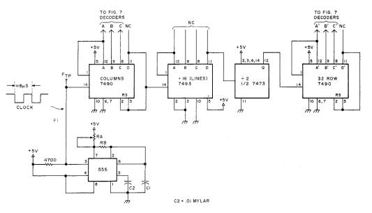
Fig. 3. Counter chain. Set for a frequency of 125 to 126 kHz at  $F_{TP}$  test point. For this application, C1 = 220 pF, Ra = 10k thumbwheel PC pot, Rb = 18k, V4-W fixed resistor. General formula is: f =  $1/T = (1.44)/Ra + 2Rb) \times C$ .
