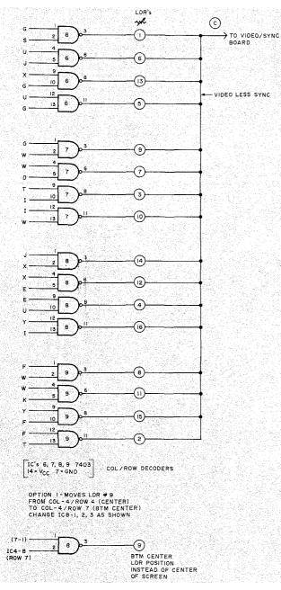
Fig. 10. Schematic of decoder board B. Option 1 moves LDR #9 from column 4/row 4 (center) to column 4/row 7 (bottom center). Change IC8 pins 1, 2, and 3 as shown, and load LDR at bottom center.
